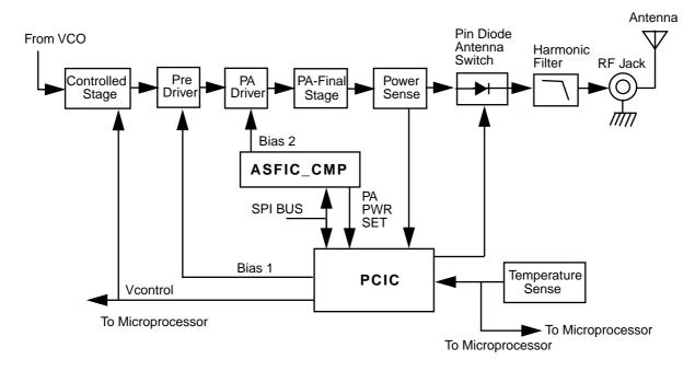
Figure 2-1 VHF Transmitter Block Diagram
