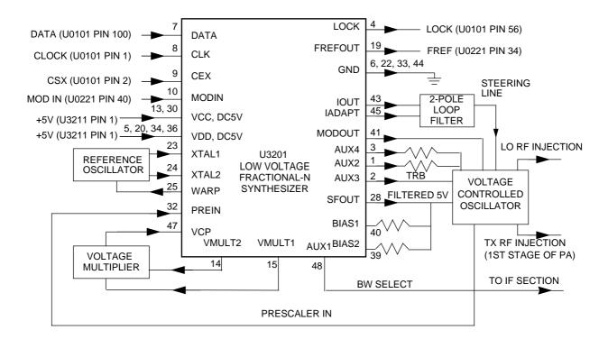
Figure 2-1 VHF Synthesizer Block Diagram
