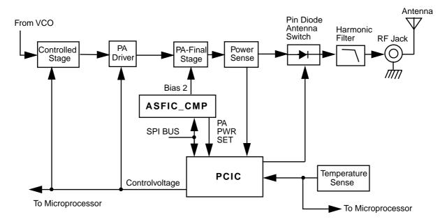
Figure 2-1 VHF Transmitter Block Diagram
