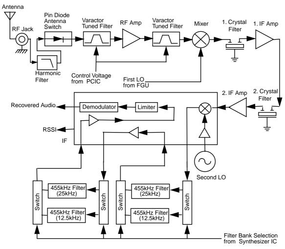
Figure 2-1 VHF Receiver Block Diagram
