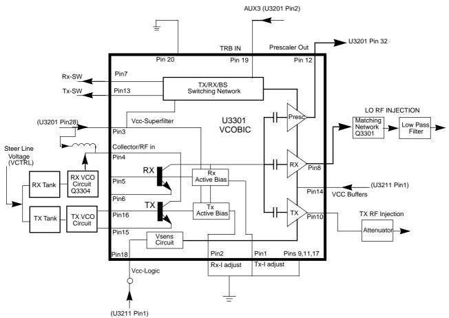
Figure 2-1 VHF VCO Block Diagram
